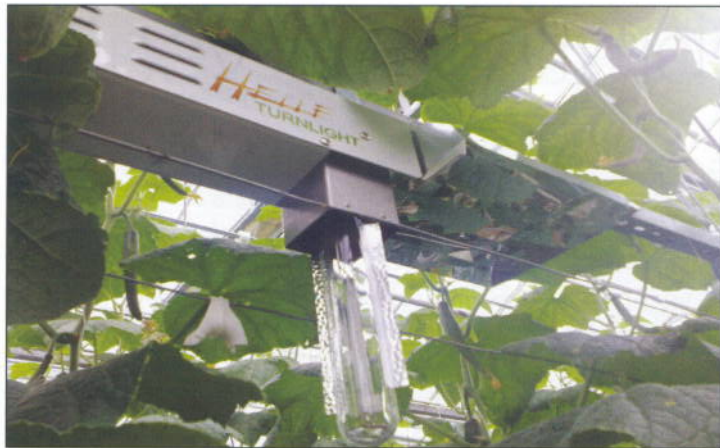
A Turnlight between the cucumbers with the lamp in the vertical position.
